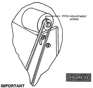
NOTE: When checking amperage with the ammeter; all louvers must be in place in the cooler; otherwise incorrect setting of the drive pulley will occur
